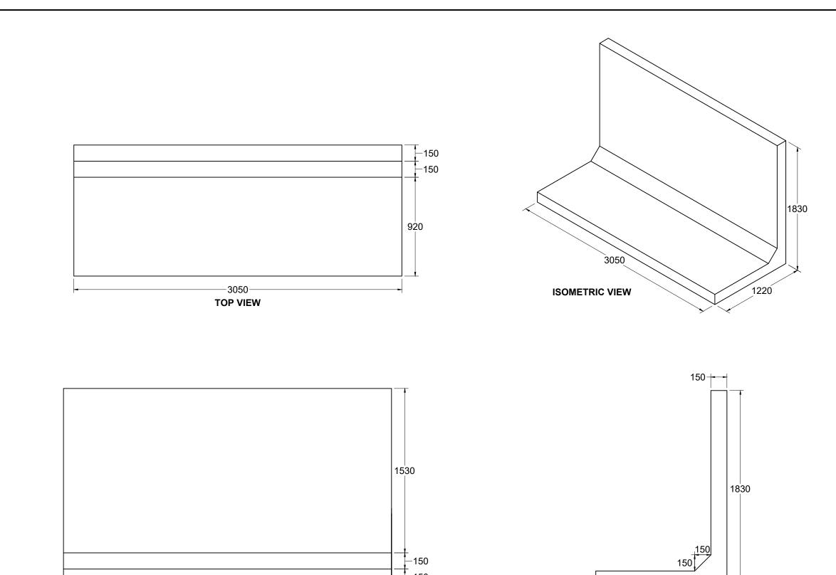
SPECIFICATIONS: PRODUCT DESIGNED IN ACCORDANCE WITH CSA A23.3 DRAWN BY: PRODUCTION: IN ACCORDANCE WITH CSA A23.4 JS 6 FT L-WALL CONCRETE: IN ACCORDANCE WITH CSA A23.1 DATE: EXPOSURE CLASS: C1, 28 DAY COMP. STRENGTH: 35MPA, AIR ENTRAINMENT 5-8% AUG 2023
