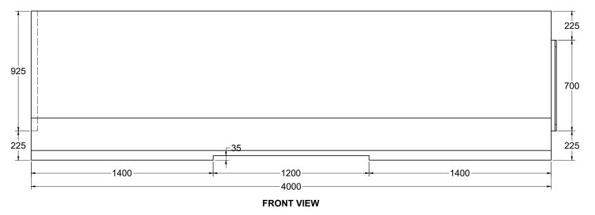
SPECIFICATIONS: PRODUCT IN ACCORDANCE WITH OPSD 911.143 DRAWN BY: 1645 SYDENHAM RD. KINGSTON, ON **TALL WALL TRAFFIC BARRIER** ANCHOR JS PRODUCTION: IN ACCORDANCE WITH CSA A23.4 PHONE: w/ I-LOCK CONCRETE: IN ACCORDANCE WITH CSA A23.1 28 DAY COMP. STRENGTH: 35MPA, AIR ENTRAINMENT 5-8% (800) 223-0012 DATE: 1-613-546-6683 AUG 2023 REINFORCING: IN ACCORDANCE WITH WITH CSA G30.18 (OPSD 911.143) WWW.ANCHORCONCRETE.COM GRADE 400W
